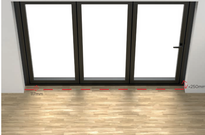
Mark 117 mm width and 20 mm depth channel on the floor close to the by-fold or patio door.
